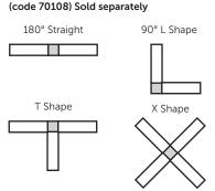
Configurations when using Link Section for Continuous Mount
